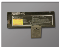
Small Sealed Lead Acid (SSLA) batteries
