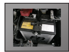
Wet Cell Lead Acid batteries
